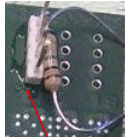
Flux from soldering operation.
