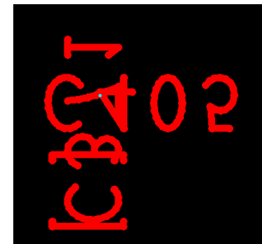
Non-legible silkscreen can be problematic during rework
